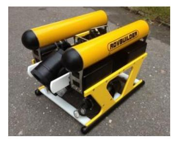
Forward Speed of the ROV RB-600 can reach up to 3.89 Knots which is equivalent to 2 meters per second
