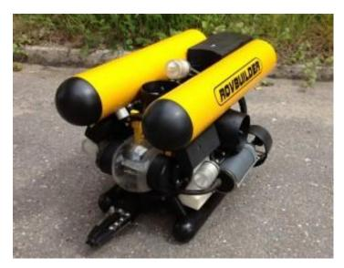
The main differences between the different models are the configuration of the thruster power, cable length, camera and depth rating.
